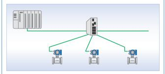
If the application requires redundancy, KROHNE's PROFINET interface can also be deployed in ring topology. In this case, the field instrument has two M12 bushings. This means that several field instruments can be interlinked via one switch integrated in the field instrument.
